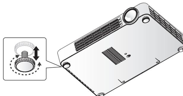
To adjust the angle of the picture, turn the tilt-adjuster right or left until the desired angle has been achieved.
